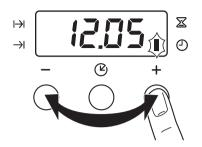
When you connect the appliance to the electrical supply or in case of a power cut, the Time function indicator flashes automatically.
